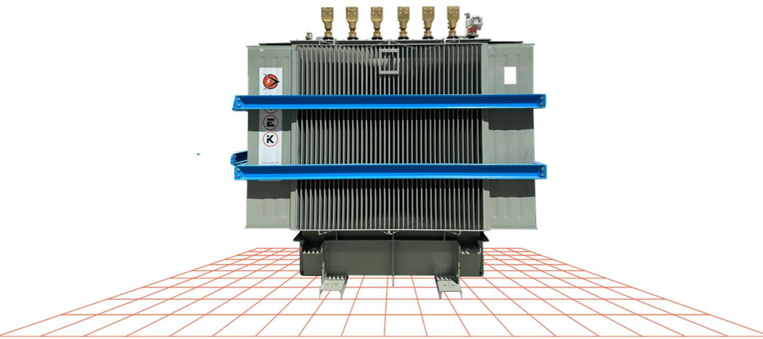
BESS transformers are designed to interface Battery Energy Storage Systems with the medium-voltage utility grid. These transformers operate in bidirectional mode, handling both charging and discharging cycles from the Power Conversion System (PCS), and must withstand frequent switching, fast transient harmonics, and nonlinear loads.
